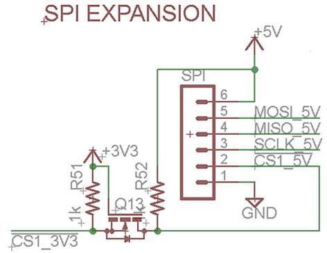
It is recommended to utilize MCP23S17 gpio expander device if a Chip Select source is needed for multiple SPI devices are desired. The MCP23S17 device is recommended due to wide usage and support provided by current Raspberry Pi distributions.
