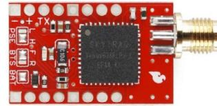
Installation of the GPS antenna requires the connectors be soldered on the **BOTTOM** of the GPS board as indicated by the silk screen.
