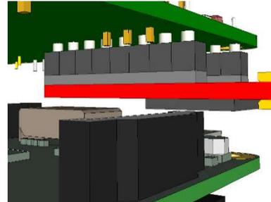
We suggest installing the pins first into the repeater board sockets, mounting the GPS board to the pins and then soldering to ensure proper alignment as the female sockets float a bit in the holes and may also be slightly angled.
