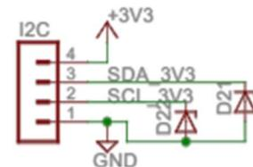
It is recommended to utilize MCP23017 gpio expander device if additional gpio functionality is desired. The MCP23017 device is recommended due to wide usage and support provided by current raspbian distributions. **Note:** Use of this chipset requires a user developed Device Tree Overlay to prevent interference with the PTT and existing GPIO expander functionality. The provided overlays only support the chipset already on-board, which is part of the repeater board's core functionality.
