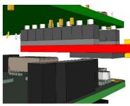
NOTE: using the GPS board is very close to the LCD flex cable socket, and may interfere with the ability to use a touch screen depending on the cable used. We have successfully folded back a ribbon cable while having the GPS unit installed, but the clearances are tight and the tight bend radius may damage your flex cable, have a spare flex cable and proceed with caution.
