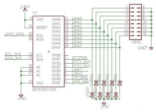
Connector Selection: Due to the tight spacing of the board, it is important to select mating connectors that do not exceed the width of the male pin alignment blocks, or you risk mechanical interference with the port 2 header. For custom cables we suggest using connector block <u>952-2037-ND from Digikey</u>, or a similar variant. **STANDARD IDC RIBBON CABLE CONNECTORS WILL NOT FIT.**
