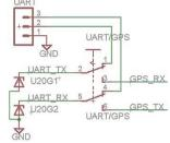
The signal levels on this connection are all 3.3V logic, and Zener diodes have been included to help protect the devices, but are intended to protect against transient voltage spikes resulting from mating connectors or similar. These will not protect again improper voltages applied to the pins.
